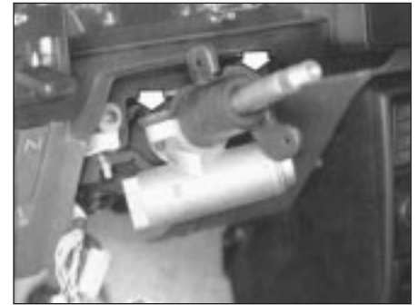
Fig. 10.9 Steering column lock shear bolts (arrowed) (Sec 9)
