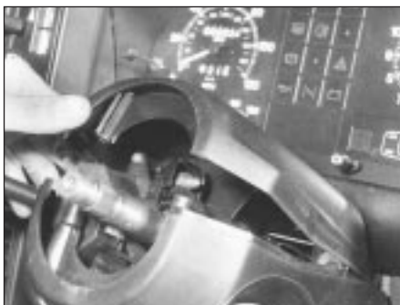
5.2 Removing steering column shrouds
