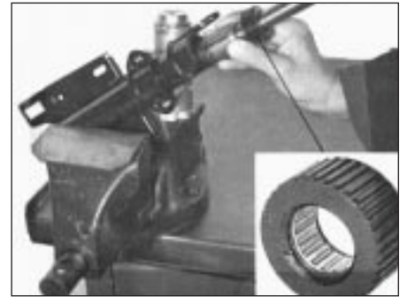
Fig. 10.4 Renewing steering shaft bushes (Sec 5)
